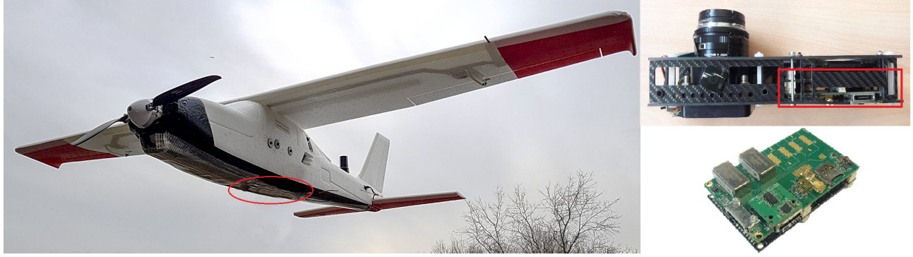
Figure 4: Fixed-wing platform with 5 control surfaces (left), PixHawk AP, precise GNSS and a payload containing DigiCAM (top-right), Gecko board (bottom-right) with two Navchip IMUs and 32-bit micro computer.
